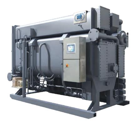
H2-type steam operated double effect lithium bromide absorption chiller is a kind of large-size industrial facility with steam as the driving energy and lithium bromide solution as the absorbent and water as refrigerant.
