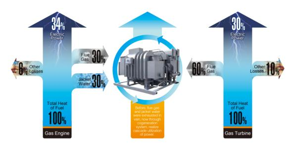
Trigeneration system can be widely used in places where electric power and air conditioning requirements exist simultaneously, such as factories, hospitals, large department stores, communities and industrial parks.
