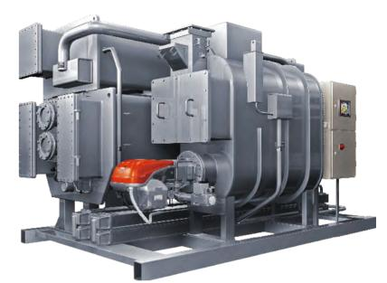
H2-type direct fired lithium bromide absorption chiller/heater is a kind of largesize industrial facility to supply cool or heat with gas (natural gas, city gas, or LPG) or oil (diesel oil) as the driving energy and lithium bromide solution as the absorbent and water as refrigerant.
