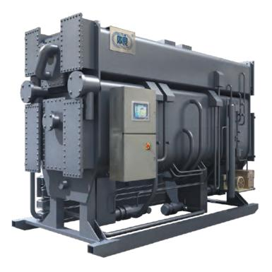
Hot water operated two stage lithium bromide absorption chiller is a kind of large-size industrial facility with hot water as the driving energy and lithium bromide solution as the absorbent and water as refrigerant.
