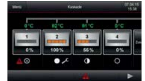
Vitotrol 350-C – default display of cascade for up to four wood boilers
